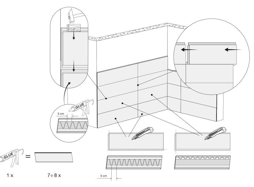
When placing the first panel on the wall, trim the tongue or the groove using a wallpaper trimming knife. When installing the panels with glue, make sure that the surface is smooth, not crumbling, ensuring good adhesion (for example: concrete, ceramic tiles, drywall). The surface of the first panel on a given wall should be completely covered with glue, each successive one only along the panel's edge with the tongue.
