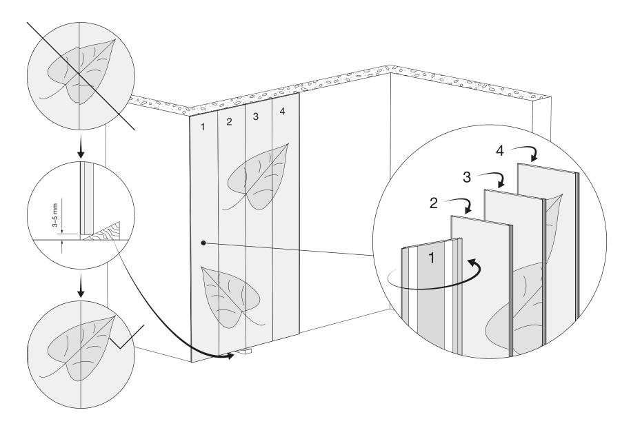
A wedge can be used to even the printed pattern and to maintain the distance on the finishing trim.
