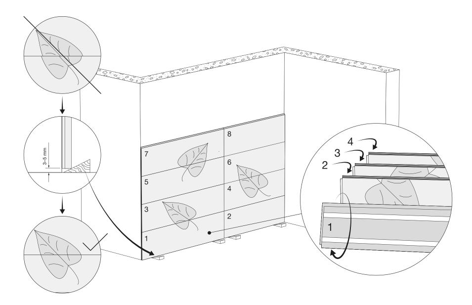
Wedges can be used to even the printed pattern and to maintain the distance on the finishing trim.
