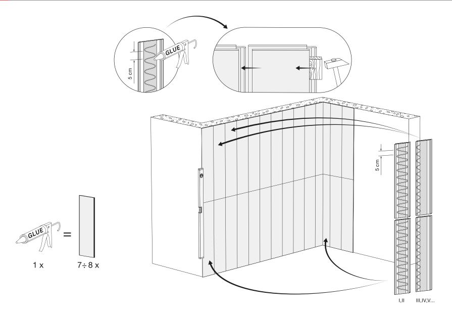
When installing with glue, make sure that the surface is smooth, not crumbling, ensuring good adhesion (for example: concrete, ceramic tiles, drywall). The surface of the first panel on a given wall should be completely covered with glue, each successive one only along the panel's edge with the tongue.
