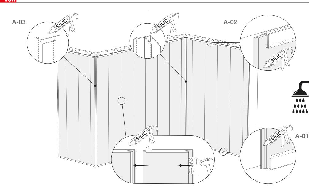
KERRADECO panels are waterproof, but their joints need to be additionally sealed with silicon – to prevent water from penetrating the gaps. Particular attention should be paid to the angles and to the spaces along the ceiling and the floor.
