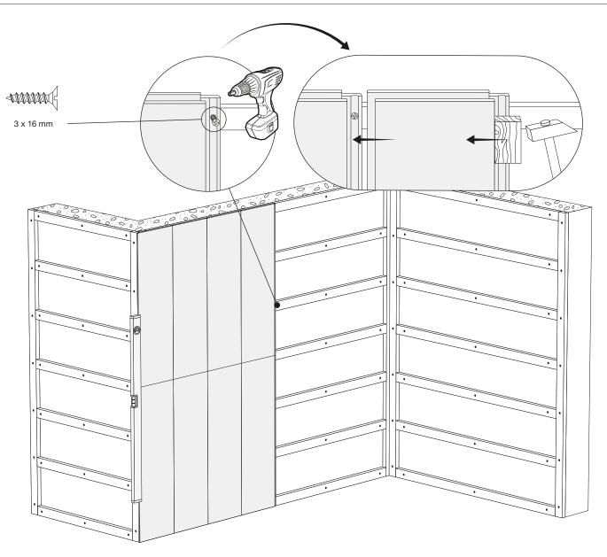
A tapping block should be used to avoid damage to the panel's edge or its groove. The panels should be placed without any gaps between them.
