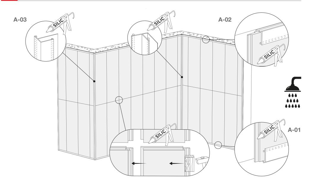
KERRADECO panels are waterproof, but their joints need to be additionally sealed up silicon – to prevent water from penetrating the gaps. Particular attention should be paid to the angles and to the spaces along the ceiling and the floor.
