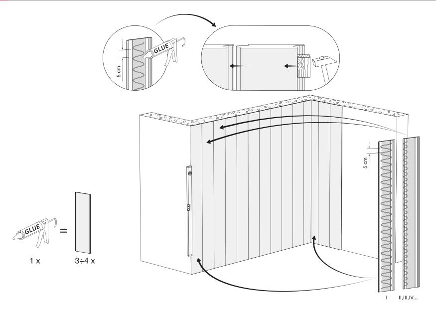
When installing panels with glue, make sure that the surface is smooth, not crumbling, ensuring good adhesion (for example: concrete, ceramic tiles, drywall). The surface of the first panel on a given wall should be completely covered with glue, each successive one only along the panel's edge with the tongue.
