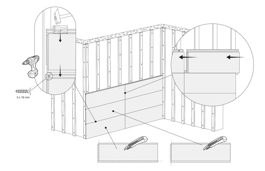
When placing the first panel on the wall, trim the tongue or the groove using a wallpaper trimming knife. A tapping block should be used to avoid damage to the panel's edge or to its groove. The panels should be placed without any gaps between them.
